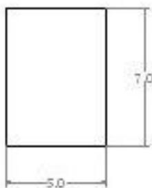
The PADD is a simple rectangle of 2mm thick plasticard. This is decorated with small pieces of 0.25mm/0.5mm thick plasticard to give the appearance of a screen and controls. I used a single screen (4mm square) and three buttons (1mm square) underneath.
